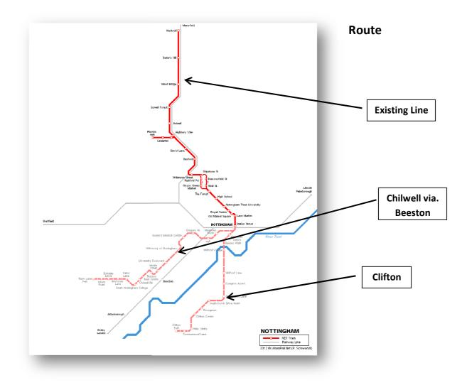
NET2 will continue south from the railway station and split into two routes, one to Clifton and one to Chilwell. The line to Clifton is 7.6km long and 63% of it is segregated. The line to Chilwell via. Beeston is 9.8km long and 59% of it is segregated. The two routes will pass through almost 40 sets of traffic signals. The overall process of planning and designing the tram route is a very lengthy process and
