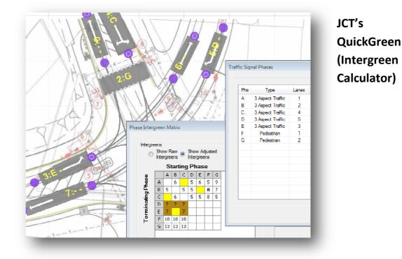
QuickGreen was found to be an excellent tool to calculate and document intergreen timings (as well as the tram calculation sheets produced specifically for NET2), and provides an auditable trail for future reference.
